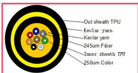
Typical cable construction for multicore cables
